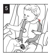
Place the child's bottom and back flat against the child restraint. This will increase comfort and allow the harness to properly tighten.
